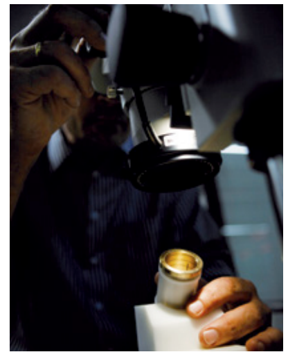
A clamping sleeve is checked for presence of burrs and chips under a microscope.
