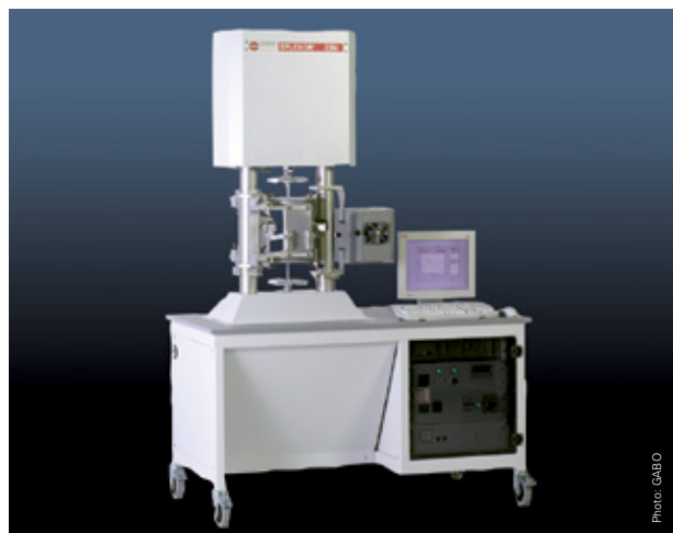
KOSTYRKA® clamping sleeves in GABO QUALIMETER test control units are operated with KOSTYRKA® air-oil hydraulic pressure intensifiers, custom-built for this application.
